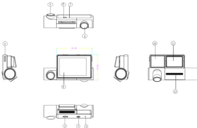
1. TF card slot 2. Micro USB port 3. Reset 4. Power
